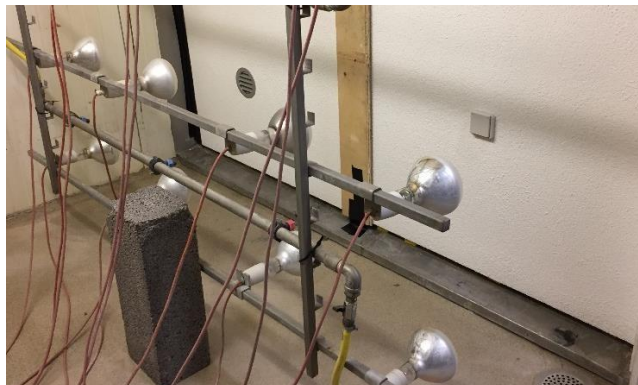
Photo 5 – Specimens during set-up for climate ageing test
